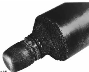
Figure 5-7. Typical Appearance of Cavitation Damage
