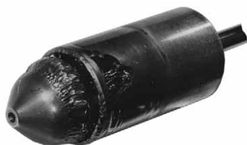
Figure 5-6. Typical Appearance of Flashing Damage
