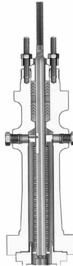
Figure 1-6. Bellows Seal Bonnet
