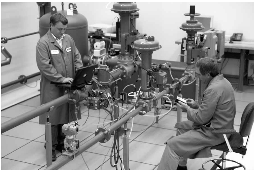
Figure 2-2. Performance Test Loop
