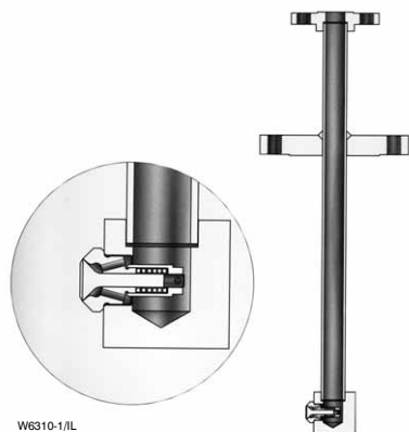
Figure 7-4. Variable Geometry Nozzle Design
