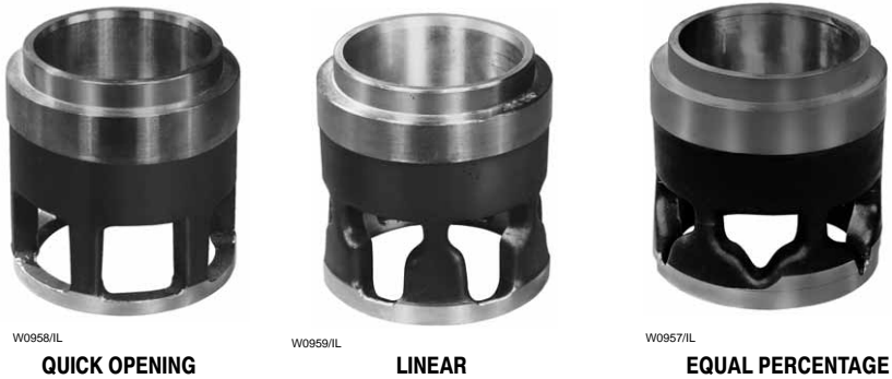
Figure 3-28. Characterized Cages for Globe-Style Valve Bodies
