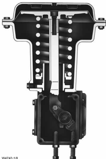
Figure 3-34. Diaphragm Actuator for Rotary Shaft Valves
