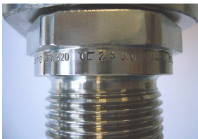
Figure 12.7.5-1: Markings of inlet body
