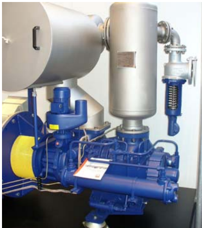
Figure 6.2.5.3-1: LESER Safety Valves in the non-upright position
