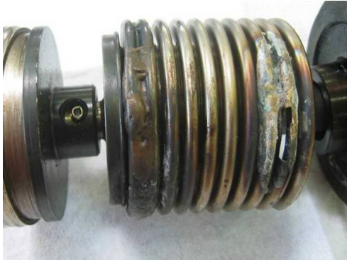
Figure 17.3.5-1: Symptom 16 - Corroded stainless steel bellows
