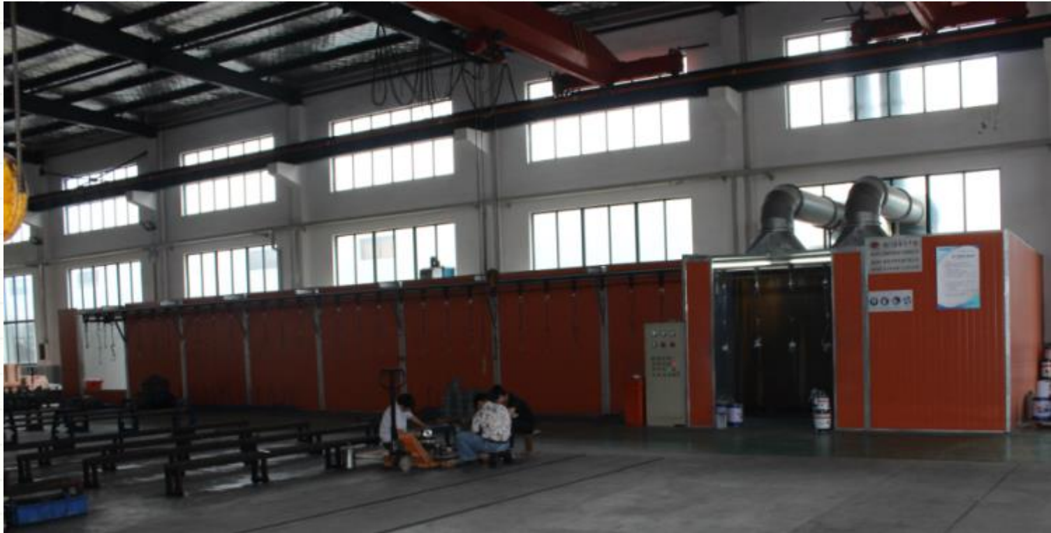
Valve painting line
