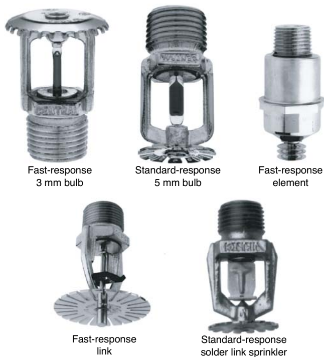
FIGURE A.5.3.1.1 Sprinkler Operating Element Identification.
