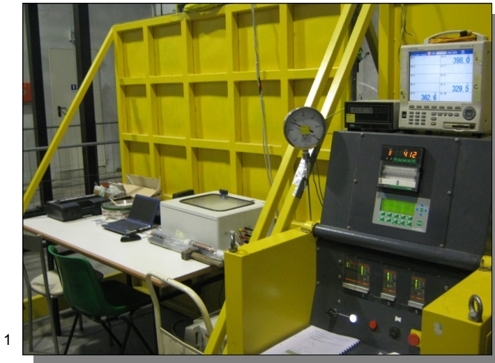
Fig.1,2 - ISO 15848-1 QUALIFICATION TEST ON PARCOL GLE 200 AND GLE 400 PACKINGS
