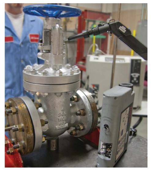
to measure and certify static and dynamic leakage values. Specific leakage rate limits for these seals are stated in VDI 2440. The values are  $10^{-4}$  mbar\*l/(s\*m) at temperatures < 250°C (482°F) and  $10^{-2}$  mbar\*l /(s\*m) at temperatures > 250°C. These leak rates must be maintained permanently.
