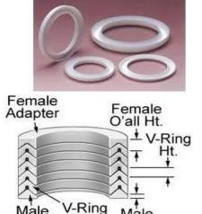
V-Packing(chevron) sealing sets are multi-part sealing sets, primarily designed for translatory movements. They generally consist of a pressure ring, a support ring and several chevron seals.
