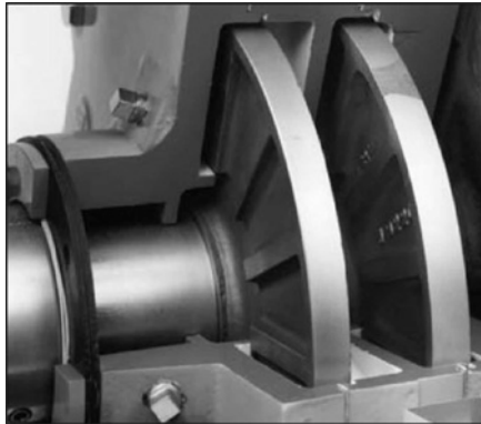
Figure 3.170 Cutaway of a centrifugal pump that is fitted with a pair of centrifugal liquid ring seals that work in series to provide the required pressure duty. (Source: Gould Pumps Inc, ITT Corp.)
