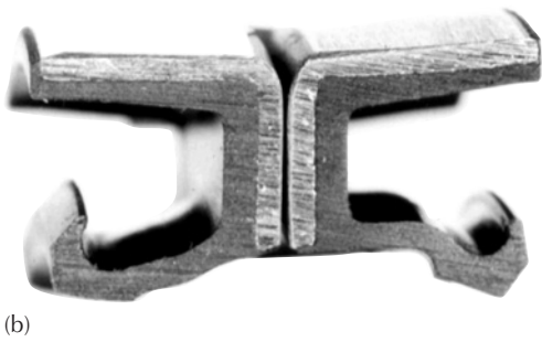
Figure 3.38 (a) Distortion of a lip seal by pressure. (b) Conventional lip seal that has been run at excessive pressure. (Source: (a) Freudenberg Simrit, (b) BHR Group)
