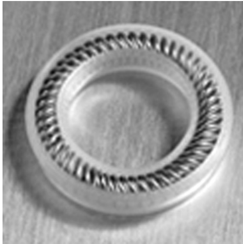
Figure 2.37 Spring energized U section PTFE seal for static applications. (Source: Balseal)
