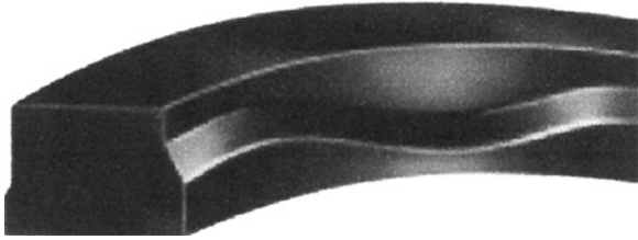
Figure 3.55 The geometry of positive lubrication seal showing the straight exclusion edge and the hydrodynamic wave for entrainment of lubricant. (Source: Kalsi)
