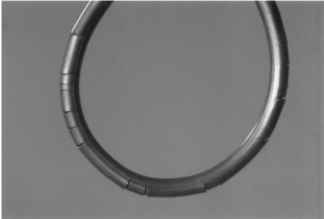
Figure 6.1 Surface cracking due to ozone attack. (Source: Freudenberg Simrit)
