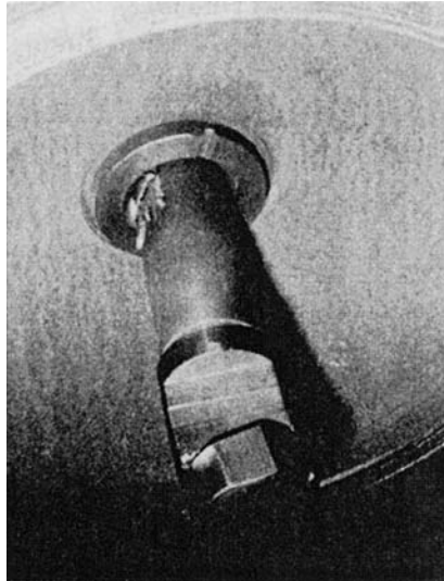
Figure 3-48. Bent Valve Stem with Damage to Stem Surface Resulting from Attempted Closure of Wedge Gate Valve with Wedge Rotated and Jammed in Valve Body, Size DN 300 (NPS 12) Class 150. (Courtesy of David Mair.)
