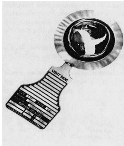
Figure 6-7. Solid Forward-Domed Rupture Disc Showing Rupture Pattern after Bursting in Liquid-Full System. (Courtesy of BS&B.)
