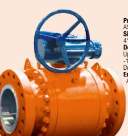
Pressure Class: ASME 150# to 1500#. Size Range: 4" to 48". **Design Temperatures:** Up to 440°C with metal seats, -196°C to +240°C with soft seat. Design API 6 D. End to End: ASME B16.10. Line Connections: ASME B16.5-B16.47, ASME B16.25. can be supplied with SR (self relieving) or DPE (double piston effect) features.
