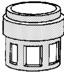
A cage with quick opening ports
