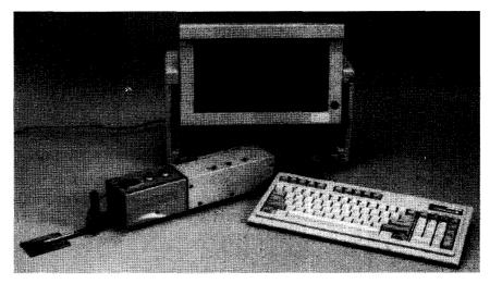
Figure 7.10 Surface finish measuring system.
