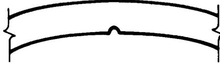
If hole is for positioning or indexing, try a small notch instead
