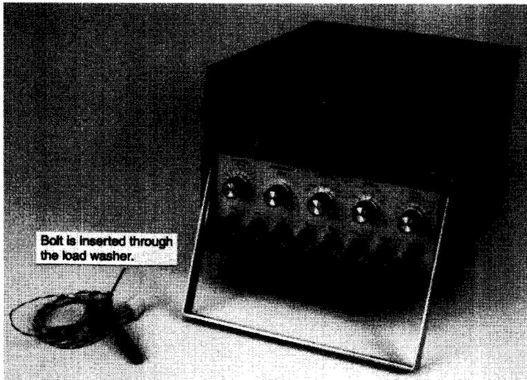
Figure 7.16 Load washer, bolt, and strain indicator.
