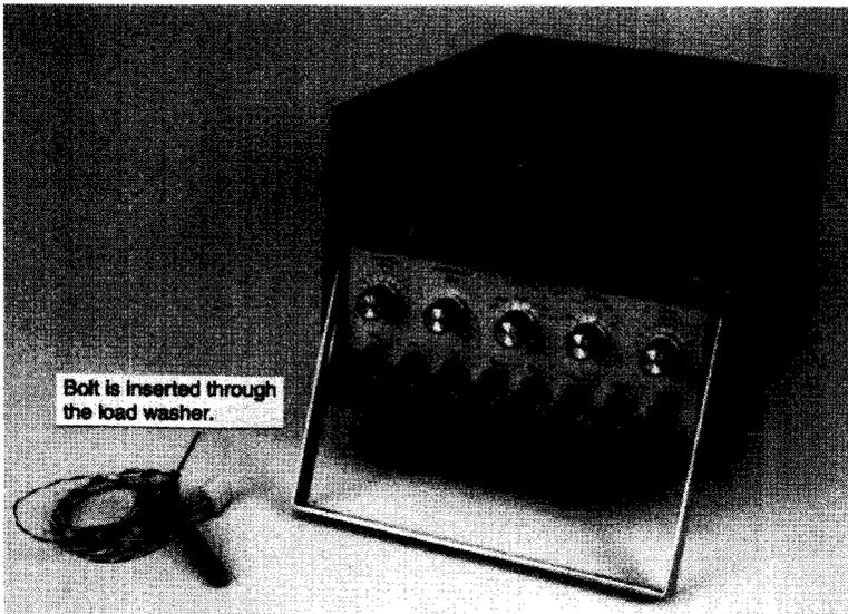
Figure 7.16 Load washer, bolt, and strain indicator.
