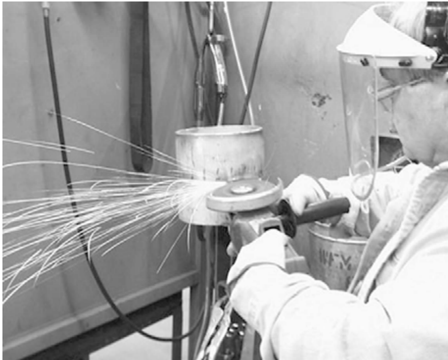
Fig. 3 Grinding of Weld Flaw
